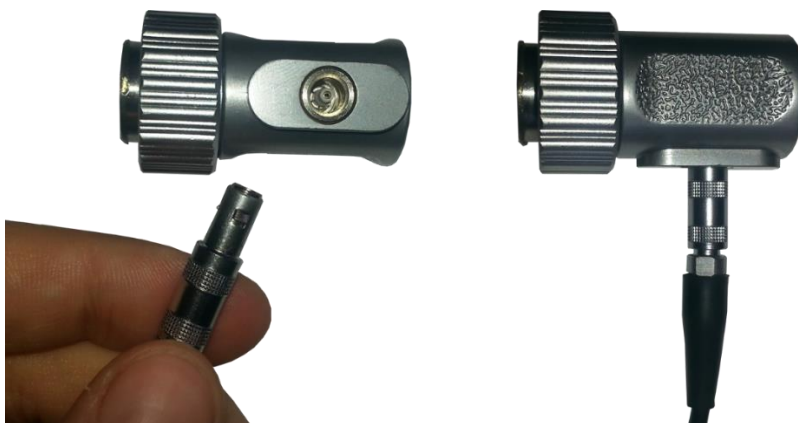
Figure 2.3 – Connecting the cable to the single element probe
