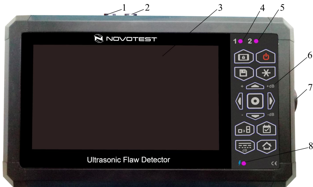
1 – port for single element probe and piezo-element output (transmitter); 2 – port for piezo-element input (receiver); 3 – colored 7-inch touch screen display; 4 – indicator of A gate; 5 – indicator of B gate; 6 – keyboard; 7 – USB port; 8 – battery indicator.
