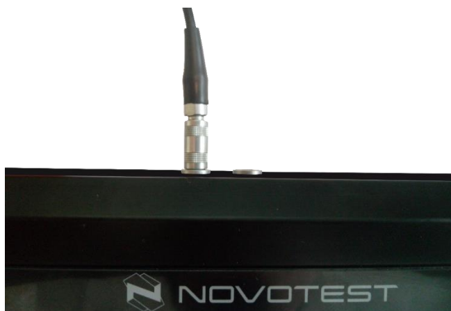
Figure 2.4 – Connecting the single element probe to the device
