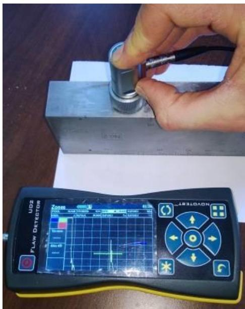
The display of device can be operated in any orientation - there are 4 options of display rotation allow user to customize the unit by himself and lefties and righties, and the instrument display can be in both portrait and landscape orientation.
