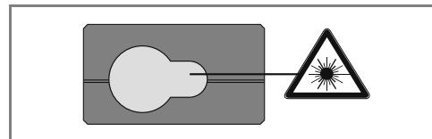
The device produces visible laser beams, which are emitted from the instrument: It is a Class 2 laser product in accordance with:
