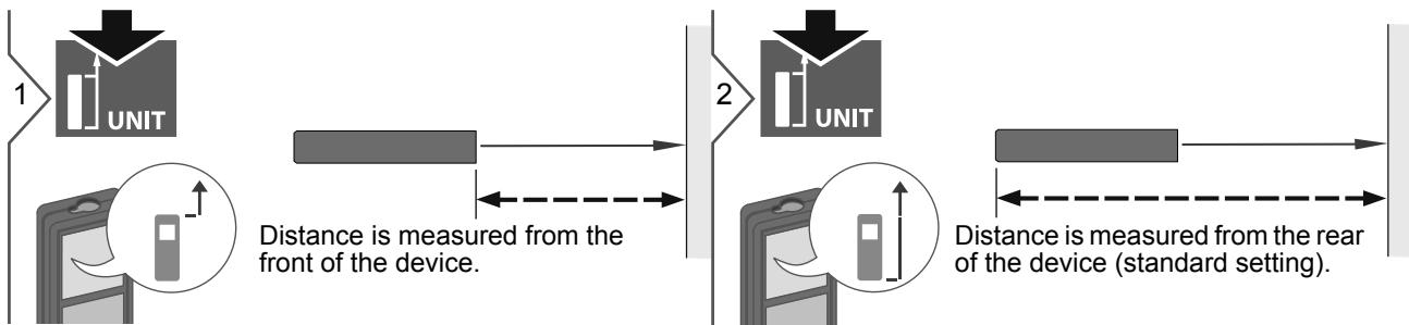
Distance is measured from the front of the device.
