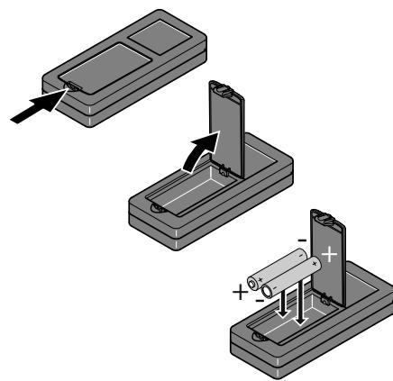
**i** To ensure a reliable use, do not use zinc-carbon batteries. Change batteries when battery symbol is flashing.
