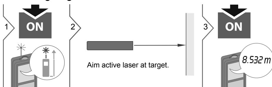
**i** Target surfaces: Measuring errors can occur when measuring to colourless liquids, glass, styrofoam or semi-permeable surfaces or when aiming at high gloss surfaces. Against dark surfaces the measuring time increases.
